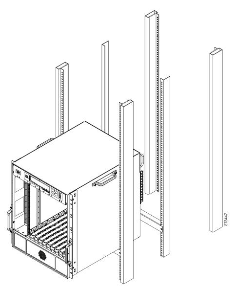
**Step 5** Remove the side chassis installation handles and slide the chassis into position in the rack.
